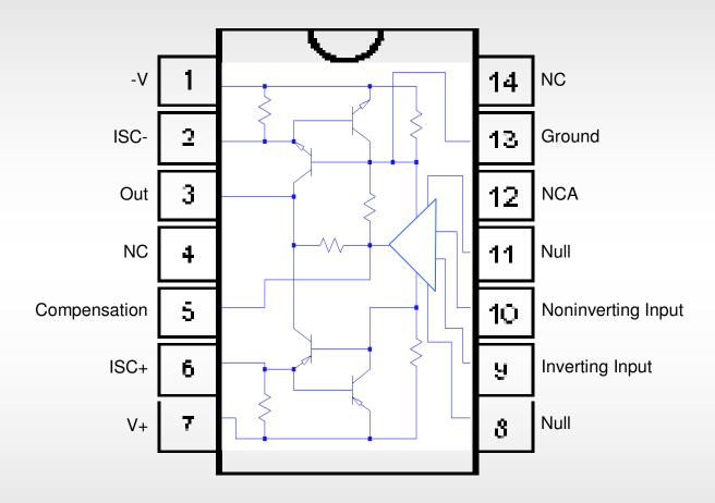
The K11 is capable of delivering large output currents not usually associated with conventional IC Op Amps. The K11 Building Block can provide up to +/-200 mA at voltage levels closely approaching the available power supplies.
